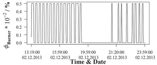
Fig. 5. Capacity percentage of boiler from measurements.
