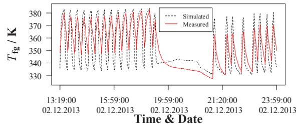
Fig. 7. Validation of flue gas temperature.
