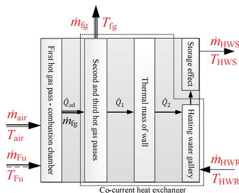
Fig. 3. Abstraction of boiler at energy center for modeling and simulation.
