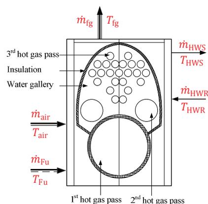
Fig. 2. Schematic showing the cross-sectional side view of the Viessmann Vitoplex 300 Type TX3 gas boiler at energy center.
