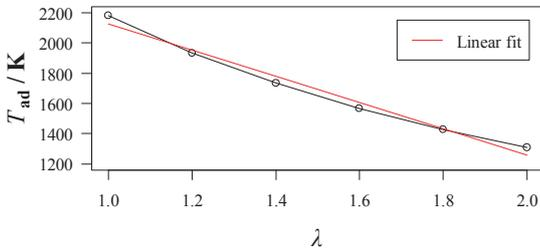
Fig. 4. Linear dependency of  $T_{ad}$  on  $\lambda$  for CH<sub>4</sub> combustion.
